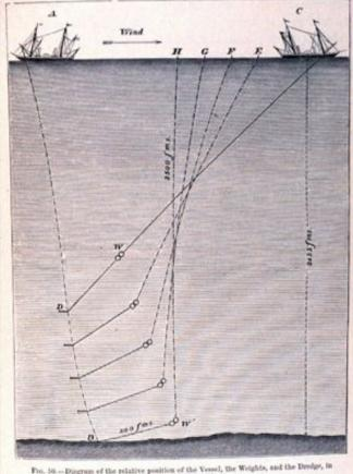
Fig. 10. -Diegram of the relative position of the Vessel, the Weights, and the best dredging in deep water.
